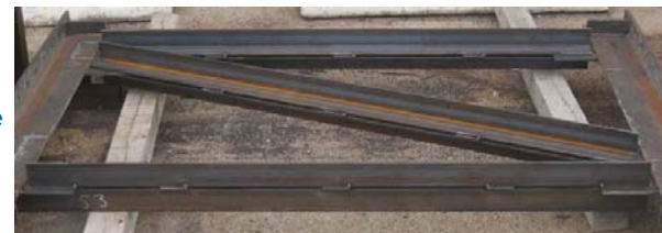
Eccentrically-loaded single angle introduces significant bending
