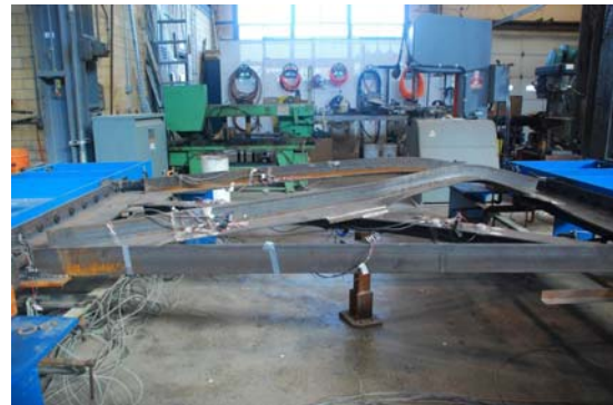
Z-type cross frame with double angle members
