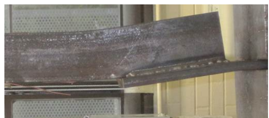
Eccentrically-loaded single angle introduces significant bending
