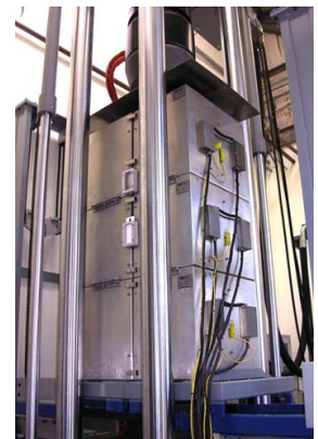
Column testing frame and furnace
