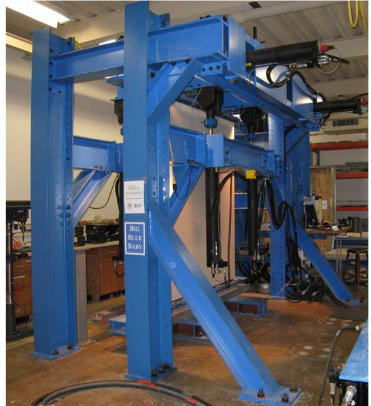
Full-scale test of cold-formed steel wall
