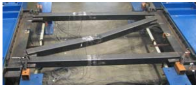
Z-type tube cross frame with knife-plate connections
