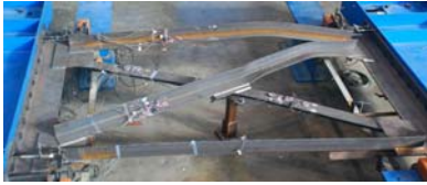
Z-type tube cross frame with knife-plate connections
